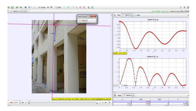
3. The default graph on the right is the displacement-time graph and speed-time graph of **mass A** as seen above. Mass A is the mass of 'bungee jump'.
